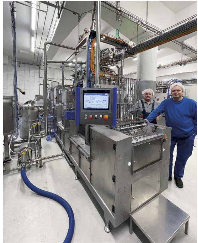
For Hügli Nahrungsmittel in Switzerland, Schuy + Folmeg supplied a filling system for salad dressing in portion packs with a capacity of 10,000 cups/h. Pictured: Dominik Mühlemann, Hügli, and Fank Orf, Schuy + Folmeg (photo: Schuy + Folmeg)
