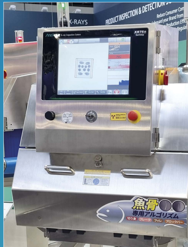
The XR75 DualX+ uses a next generation Photon Detector technology (photo: Anritsu)
