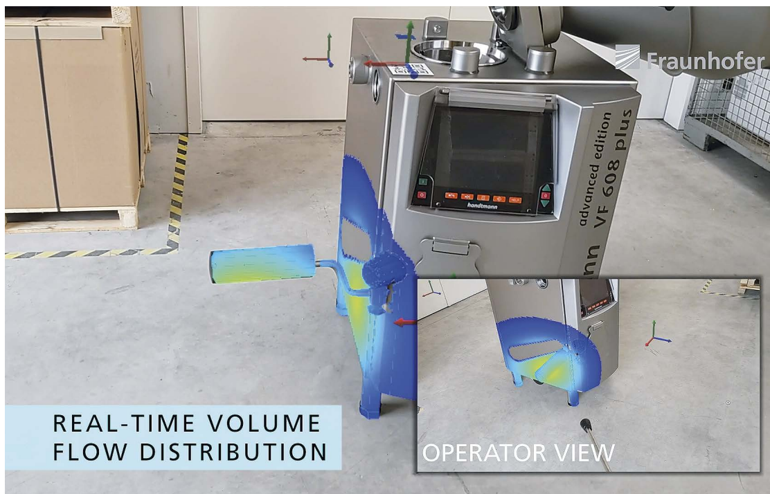
Fig. 3: Parallel live view of the AR headset with superimposed view of two employees and representation of the volume flow distribution
