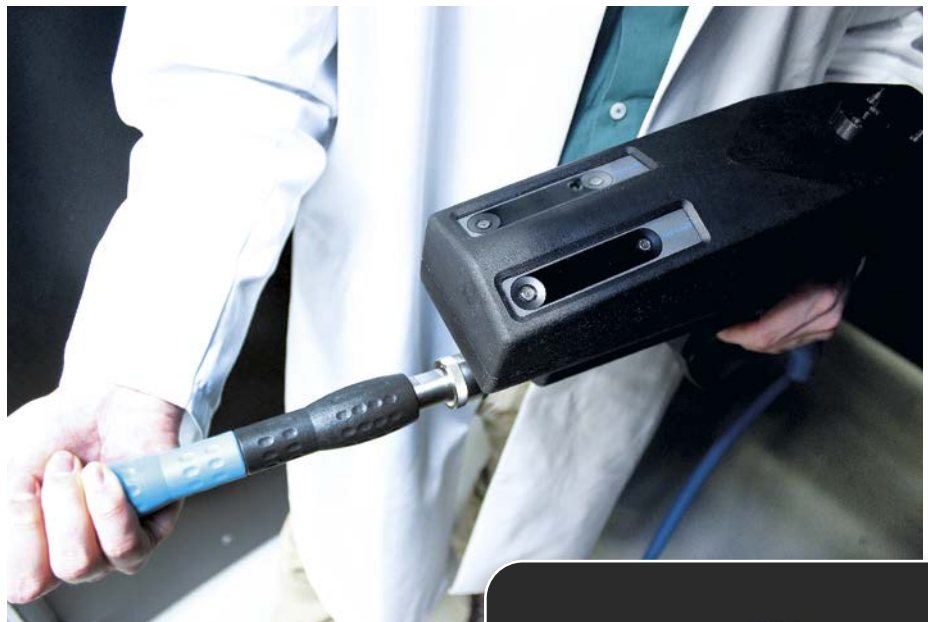
Fig. 1: Spray lance with highly integrated position and orientation tracking system (prototype)
