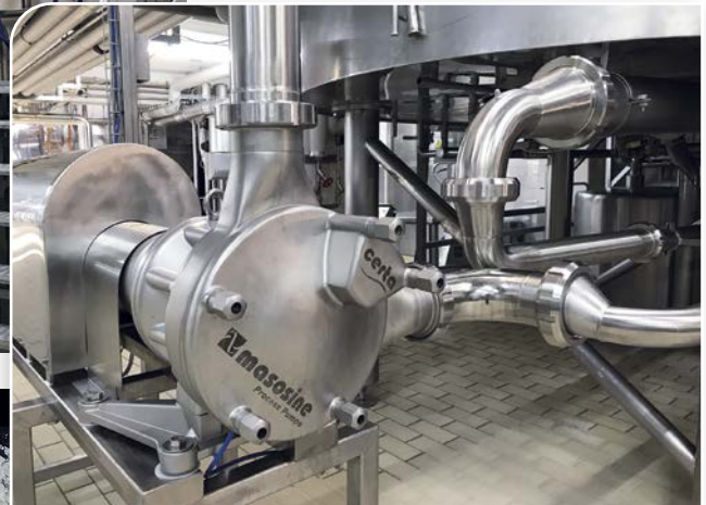
The Certa Sine pump during tests as Emmi pumping curd from the cheese vat to drain table
