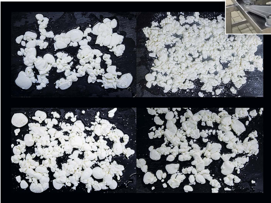
Curds after pumping: Sine pump top left, air operated diaphragm pump top right, centrifugal pump bottom left, twin-screw pump bottom right
