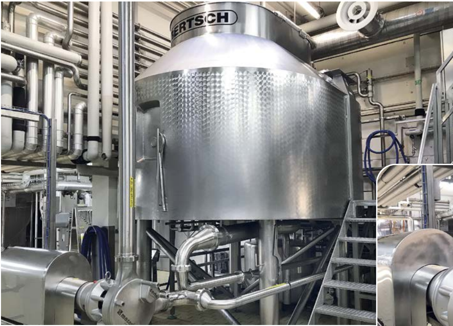
The Certa Sine pump during tests as Emmi pumping curd from the cheese vat to drain table
